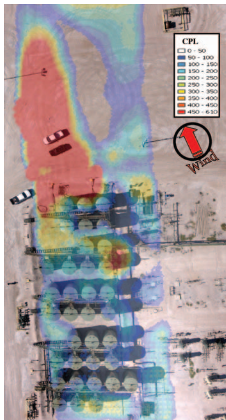
ANGEL Service report showing hydrocarbon emissions from condensate tanks. Plume concentrations are clearly defined and integrated with aerial imagery.
